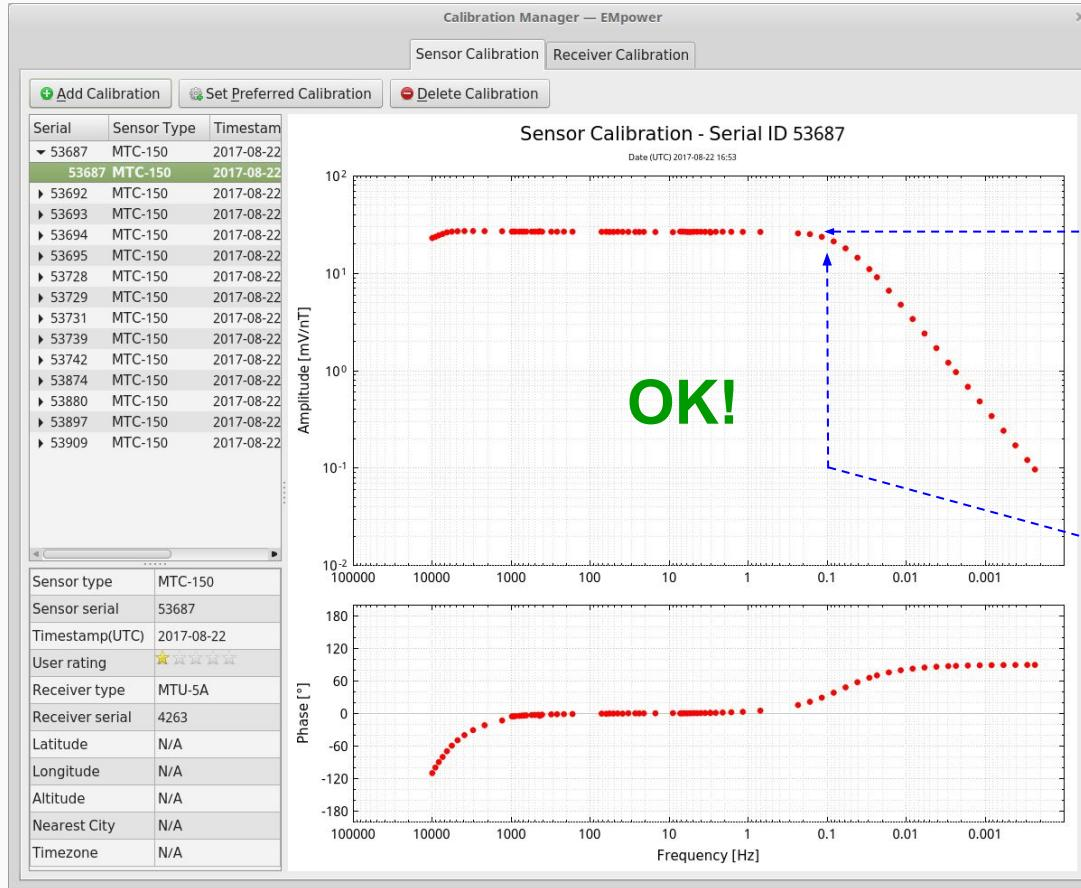
For MTC-150 the value of the horizontal part should be between 20-30
